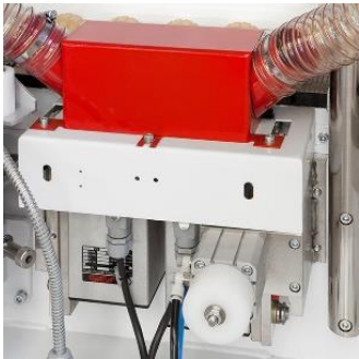
Unitate de pre-frezare Putere: 0.75 +1.1 kW.
